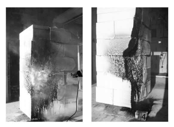
Figure 1. Flame retarded (class E) EPS during and after flame impingement with gas burner.
