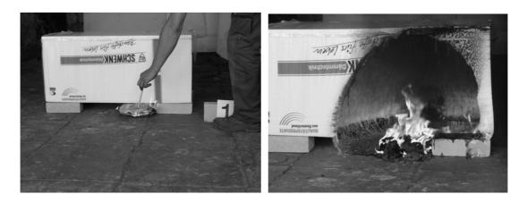
Figure 2. Paper cushion ignited below stored EPS – Melting but no continuous burning of EPS.
